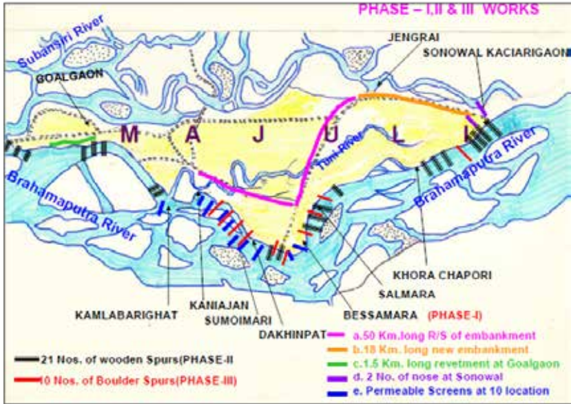
Figure 6: Locations of original embankment and different types of anti-flooding and bank erosion works carried out in Majuli by the Brahmaputra Board in Phase I, II and intended in Phase III.
